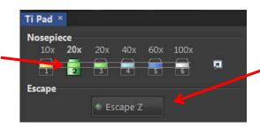
Remember to use the Escape Z function when loading and unloading your sample.
