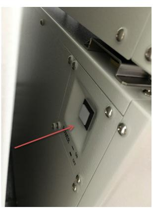
4. Turn on the two power buttons on Nikon halogen lamp (for visual diascopic microscopy).
