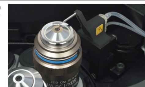
Dual micro nozzle geometry automatically keeps the proper amount of water on the tip of water immersion objectives.
