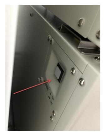
3. Turn on the power strip underneath the microscope.
