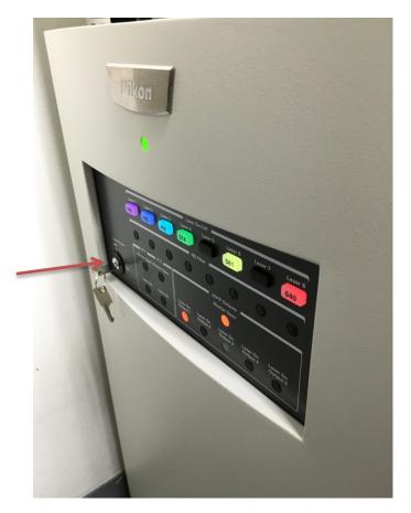
2. Press the button the left side of the A1Rsi Controller unit.
