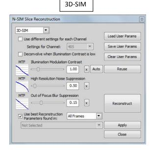
**Deconvolve when Illumination Contrast is Low:** Compares high frequency, moiré diffraction components against image noise
