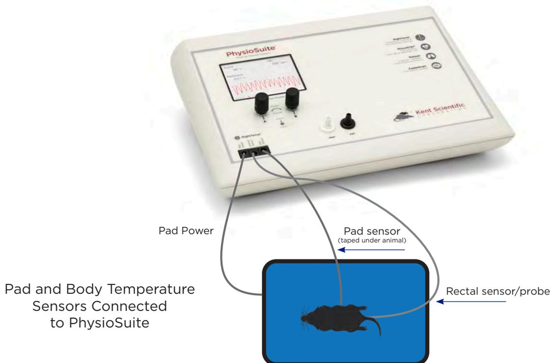
**We recommend that you secure the pad probe to the warming pad using tape, etc.**
