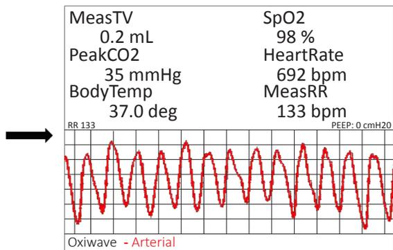
**Small text on the run screen displays the assigned Parameter name for each Dial, if set, and its current value.**
